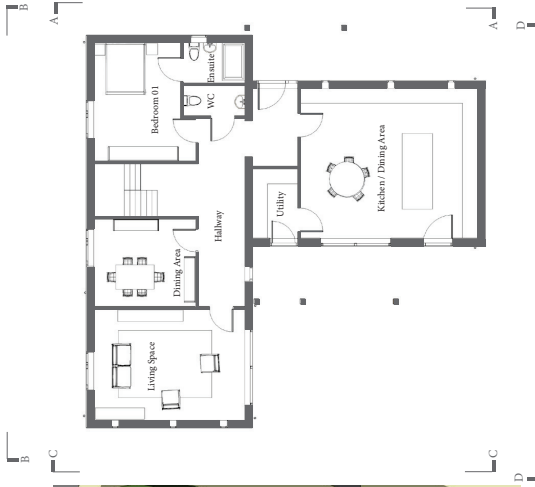
Ground Floor Plan 1:100@A1
